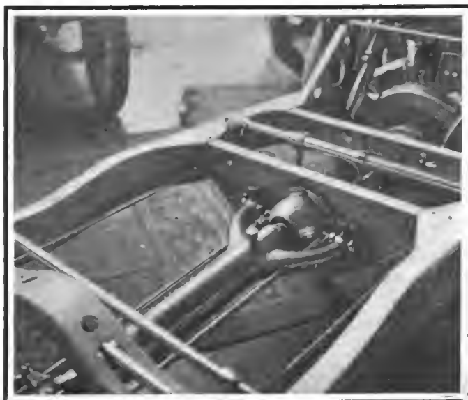
Stearns presenting details of the anchorage of the torsion tube to the cross member, presenting a large spherical bearing, universal action and the method of spanning the universal joint, which results in double bearings symmetrically disposed
